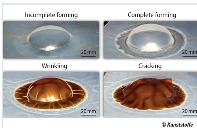
**Fig. 2.** Thermoformed polyamide 12 semi-finished products: sample parts to illustrate the thermoforming studies
