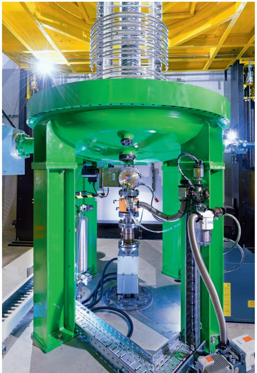
Radiation source: an electron accelerator of 3 MeV maximum energy, operated by BGS Beta-Gamma-Service at its Wiehl site near Cologne, Germany. Electrons released from a hot cathode are collimated into a beam and accelerated via alternating electric fields (© BGS/M. Steur)
